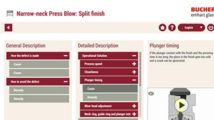
Fig. 1: The Defect Animation Tool – the electronic defect database on the UC2 and Flex Control Center
