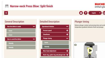
Fig. 1: The Defect Animation Tool – the electronic defect database on the UC2 and Flex Control Center
