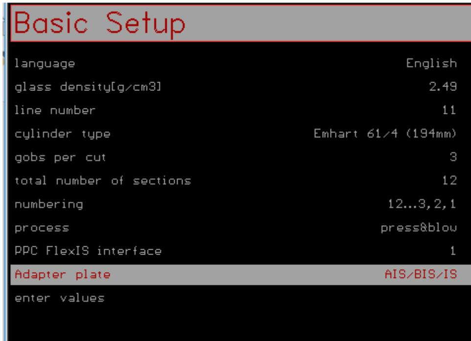
**Please be aware** that when the software is installed, you must select the correct adapter plates! Selecting “n.a.” means that the former temperature correction is used, this is not recommended! Select either “AIS/BIS/IS” or “NIS”.
