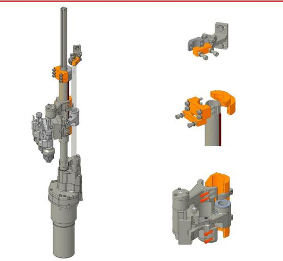
Redesigned Mounting Parts for Pantograph Baffle
