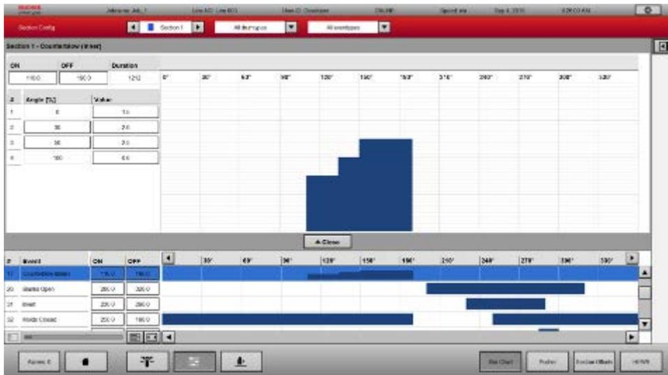
The same is possible for all section servo axis. You can adjust the position, motion duration and ramp settings directly in the bar chart.
