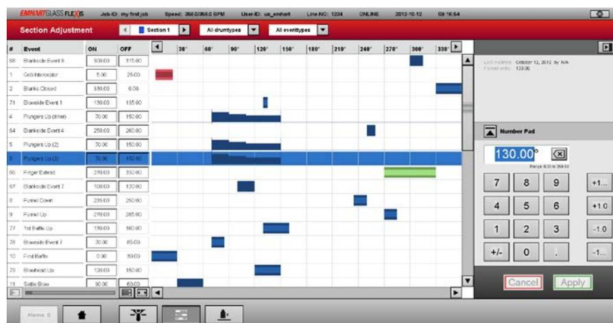
By clicking on the bar you get a detailed view of the FPS pressure settings and its corresponding timing values. All FPS settings can be made in this screen.
