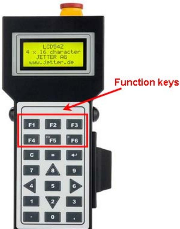
This terminal is a 4 line display equipped with a pushbutton wired on the MS circuit of the cabinet.
