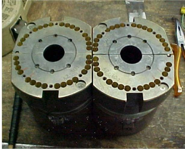
**Figure 3 – Diffuser exits implemented on a mold**
