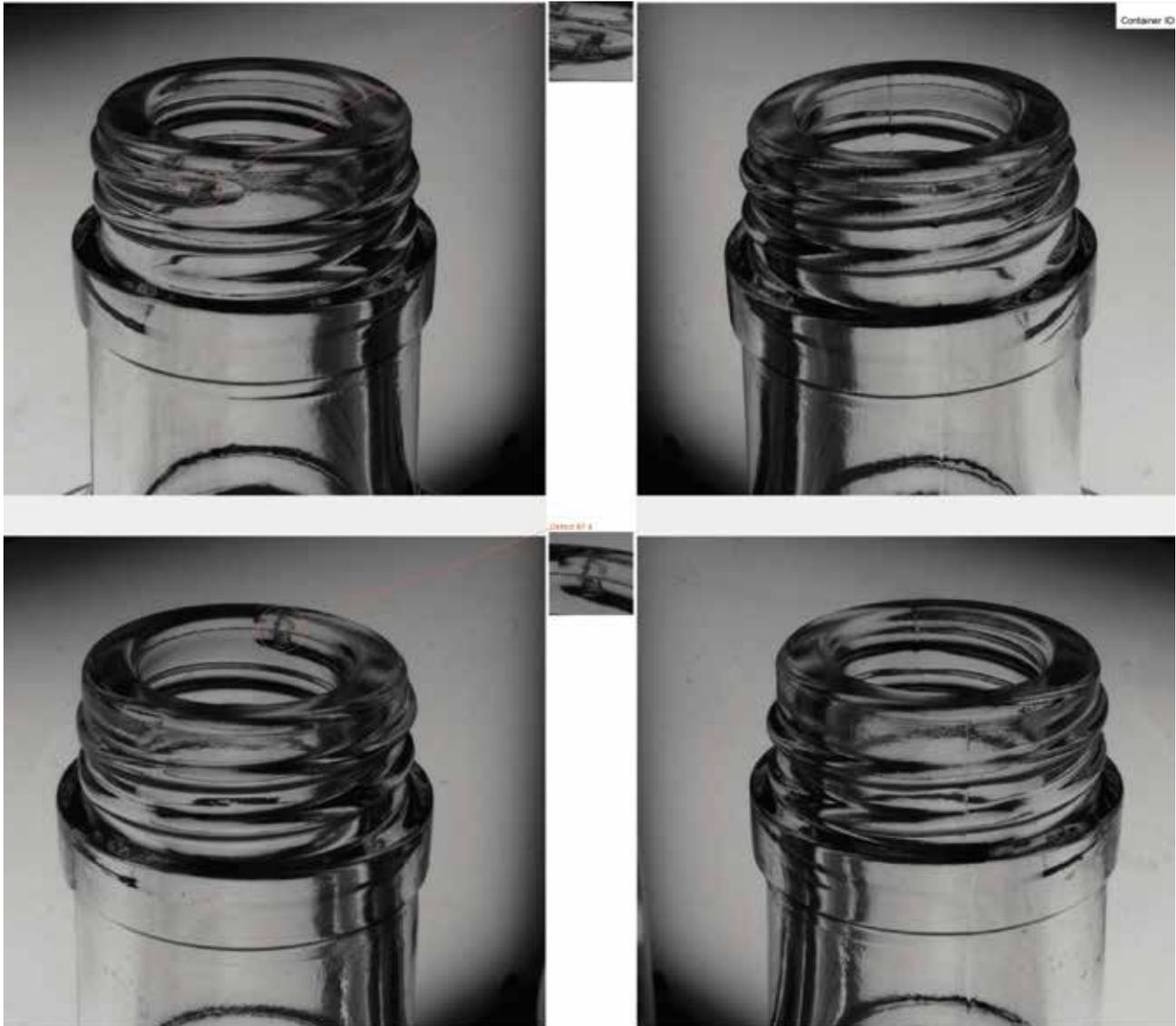
those refraction 'shadows' change over time, as the thread shaping and annealing process change.
