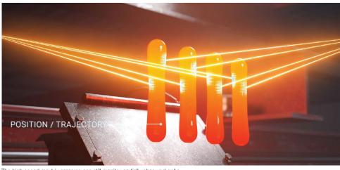
The high speed maxtrix cameras can still monitor partially obscured gobs.
