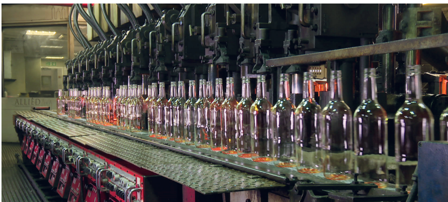
▲ The BIS can handle a wider variety of container designs, sizes and weights.
