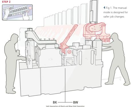
job change on a glass-forming machine is always a challenge. Each minute without glass has an economic impact on the plant. Therefore, diminishing the downtime is a key goal. To optimise the machine shutdown, there is a high level of co-activity on the machine, with operators working simultaneously on both sides of the machine. Numerous parts of the section equipment have to be changed and adjusted.
