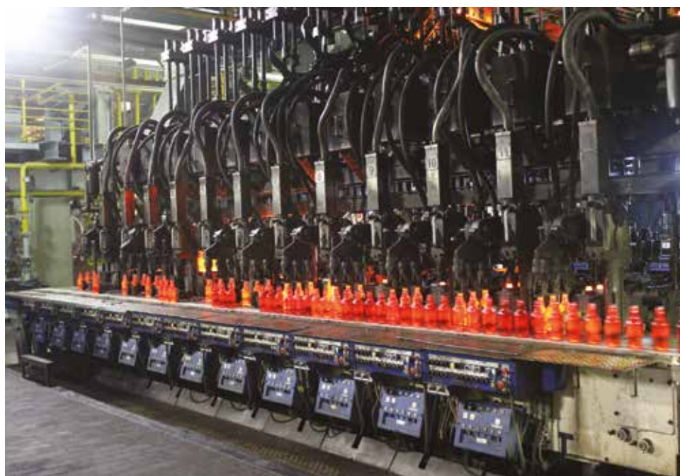
Each production line in Vidroporto's third production shop is equipped with a Bucher Emhart Glass 12-section triple gob AIS forming machine.
