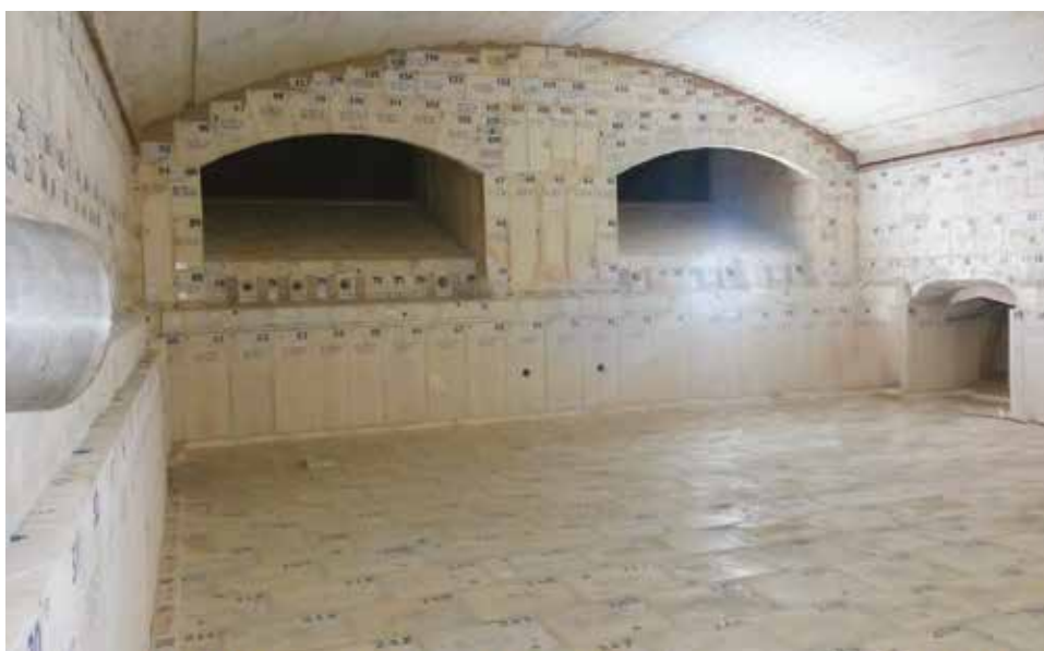
The furnace has been provided by HORN Glass Industries AG and can produce on average 42 million bottles/month or 350 tons of glass/day.
