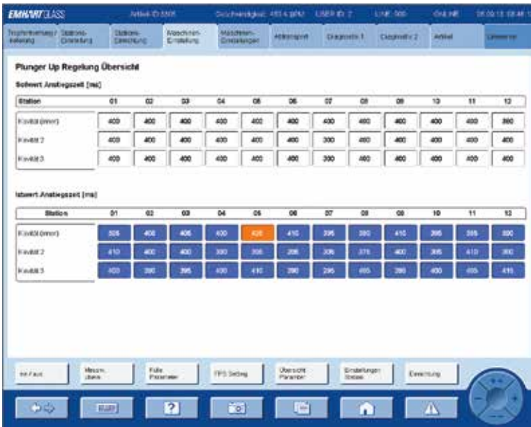
Overview page of the FlexIS Plunger Up Control, showing setpoint and measured values. The background colour indicates all cavities switched on and cavity one of section five operating at the allowed pressure limit.
