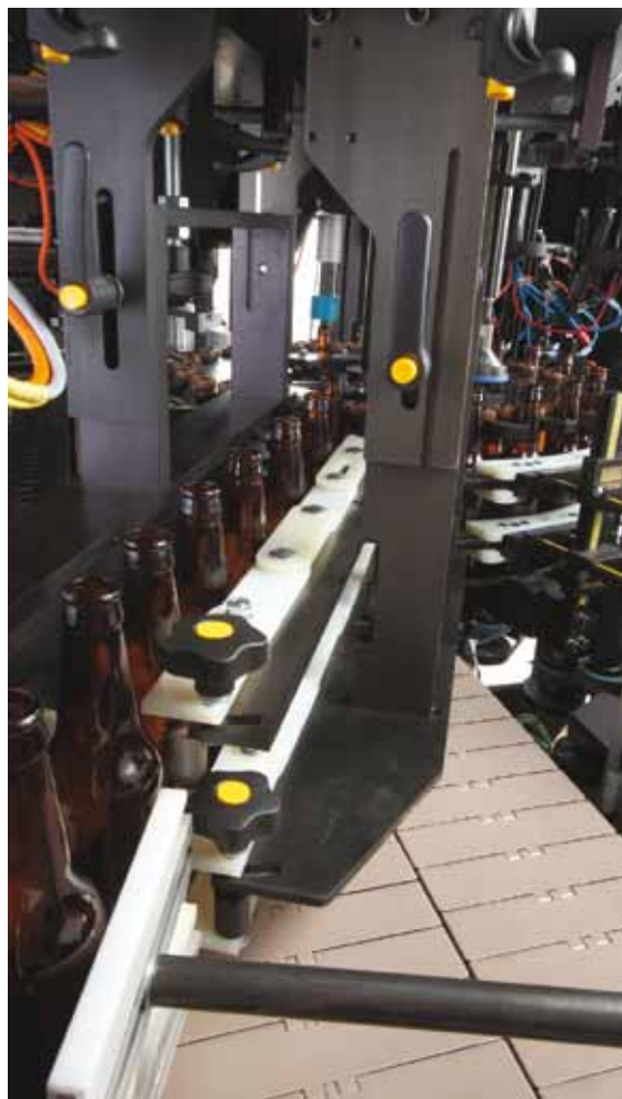
Infeed screw of the recently introduced Type M machine. The 30° angle enables stable container handling.
