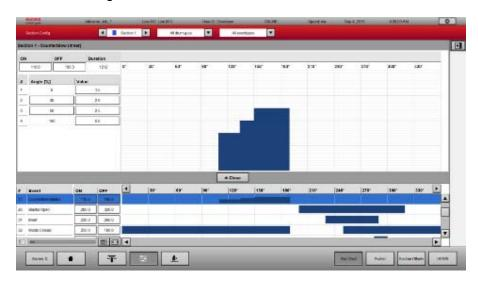
The same is possible for all section servo axis. You can adjust the position, motion duration and ramp settings directly in the bar chart.
