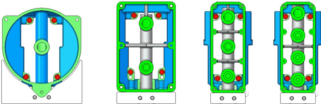
The vacuum tubes are now removable for cleaning purposes in DG, TG and QG configuration for an improved maintainability and higher mechanism efficiency. The same screws secure the distributor plate and the vacuum tube. Once the distributor plate is out, the vacuum manifold is free to be removed without the needs of tools.
