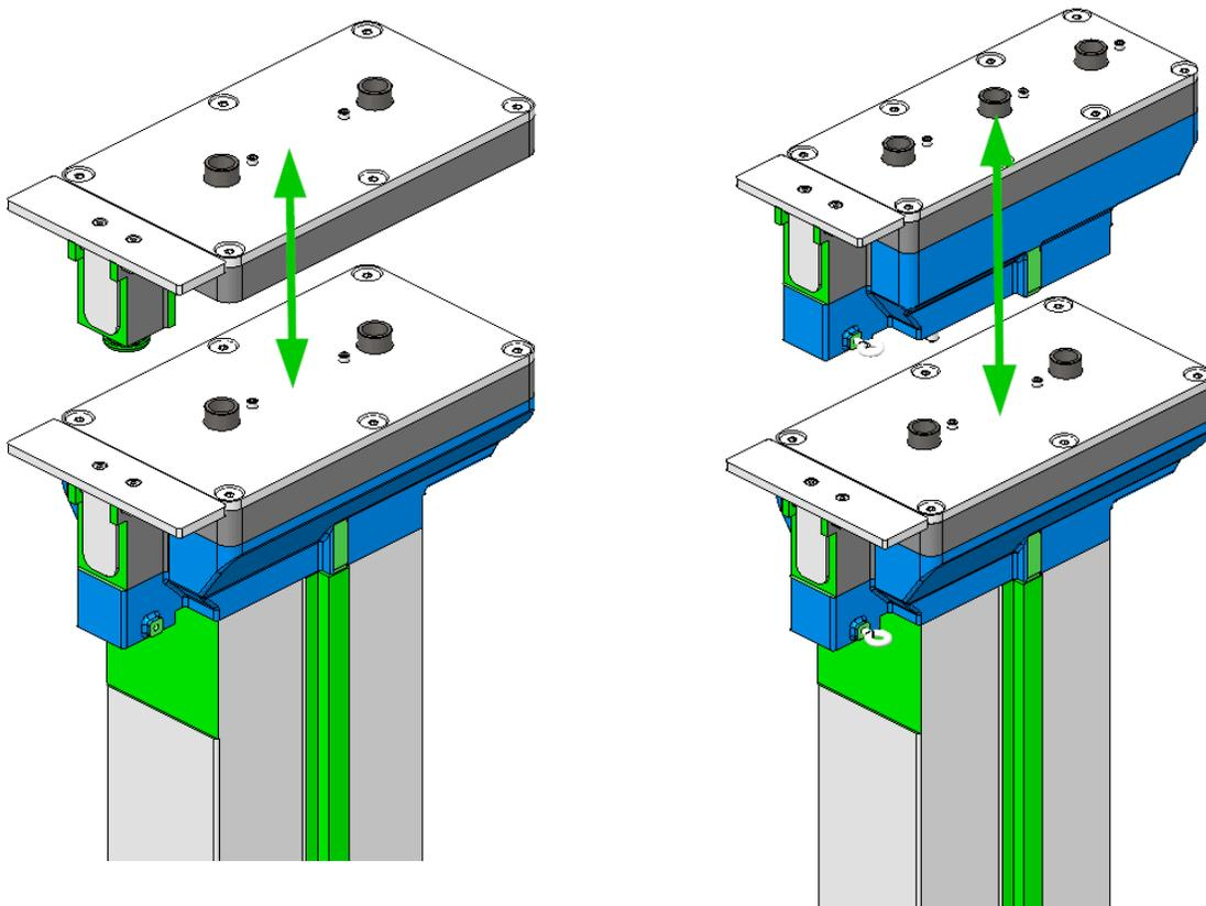
For converting the machine from SG to DG or TG the upper bracket has to be replaced. After the distributor plate removal, the screws which are fastening the upper bracket to the lower bracket are easily accessible for a fast conversion.
