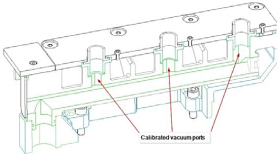
Vacuum flow for each cavity is equally balanced by a specific porting in the vacuum ducts.
