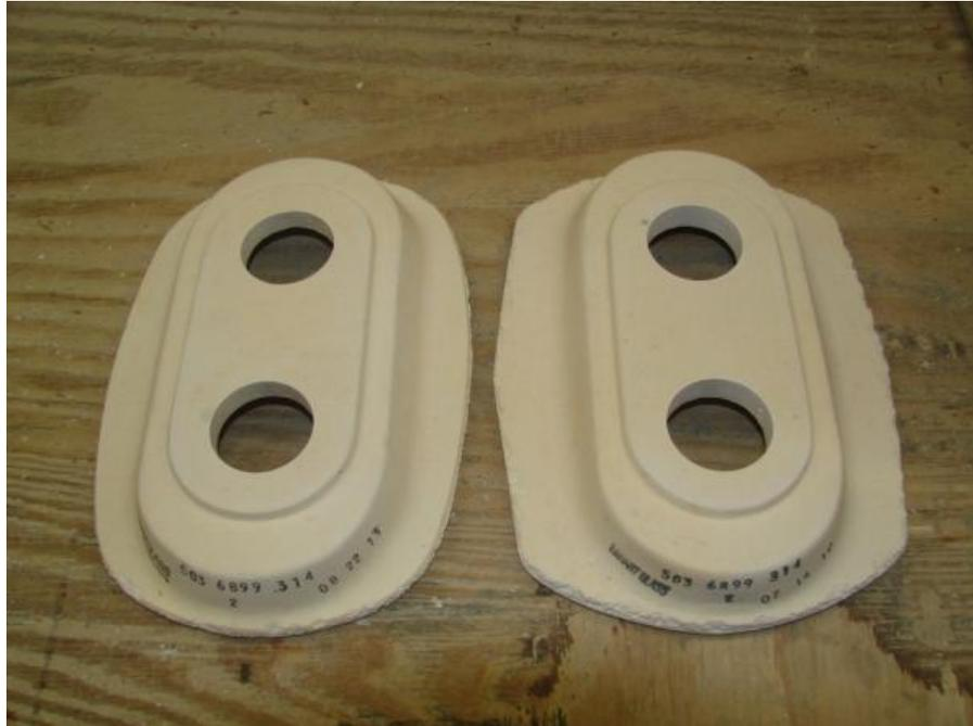
*515 Metering Orifice Rings of the new style (left) and old style (right).*
