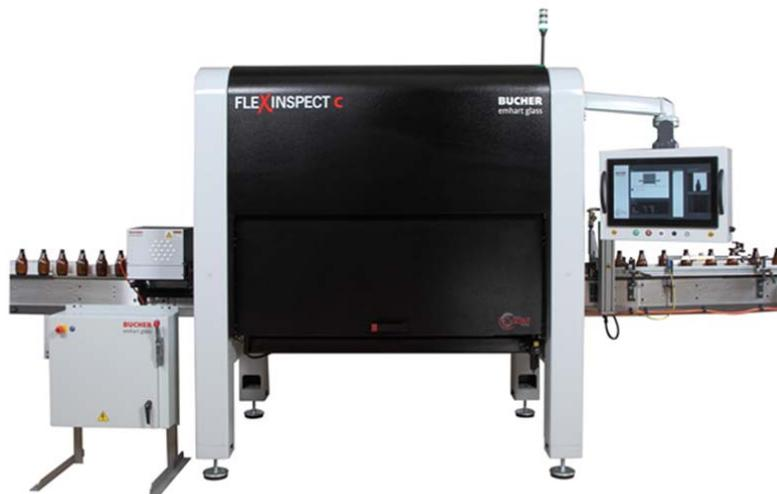
The FleXinspect C is designed to inspect round and non-round glass containers at speeds up to 600 containers per minute.
