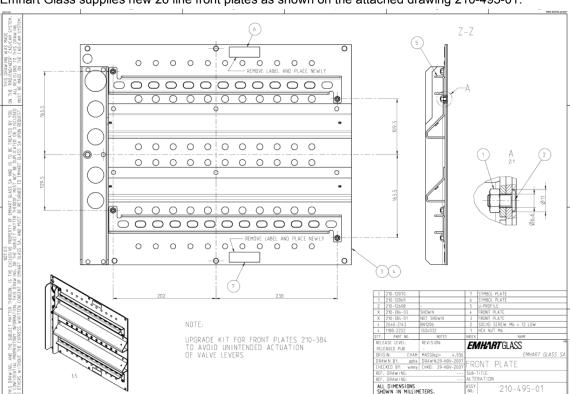
Emhart Glass supplies new 26 line front plates as shown on the attached drawing 210-495-01.
